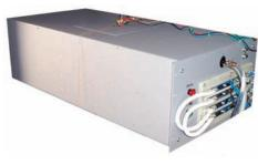
A self contained 32KW power system with fans and heat exchangers to provide internal cooling. This 10" X 17" X 36" enclosure contains four 8.1KW AC/DC power supplies with the AC fed through the top and DC output bus bars on the front and rear. A power on button and EMO stop on the front panel for external control and an RS485 communication port for monitoring.
