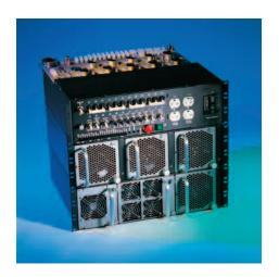
This contains four AC/DC switching power supplies, one linear power supply, and one high voltage power supply (325V). An extensive AC and DC distribution system with numerous circuit breakers, a main contactor and an EMO safety circuit.
