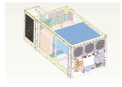
A 32KVA isolation transformer with taps for three different input voltages was required for this Field Replaceable Unit. The 15KW of 48V redundant power was supplied by four 5KW AC/DC power supplies.
