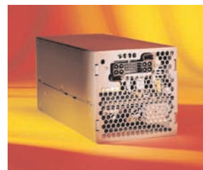
5" x 5" x 11.5" Up to 3000W Elcon lower Drawer Hot Plug Connector
